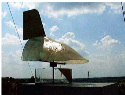
Figure 36 Rotating cowl developed in Photovent project
